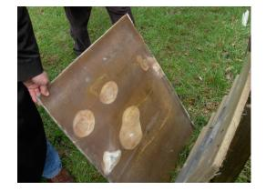
The lower left corner of the photo shows the panel shot by a 12 gage shot gun with number 4 shot. This was repeated nine times. The panel was shot from a distances of 15 feet. The upper left corner of photo reflects three hits from a 38-caliber revolver. The distance to the panel was 10 feet. The upper right center of the photo shows five shots from a 357 magnum at 15 feet. The photo of the rear of the panel shows no penetration by any of the shells or pellets.
